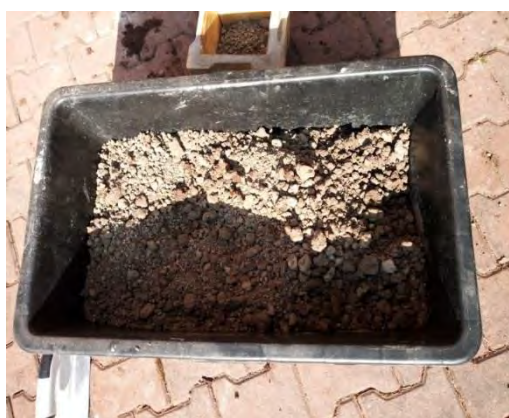
Fig. 1. Mixture of soil and cement
