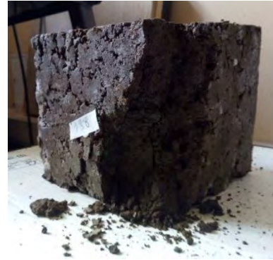
Fig. 3. Mechanism of destruction of soil-cement composite
