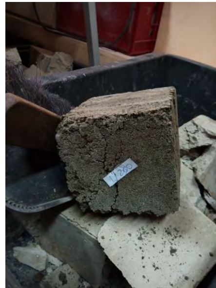
Fig. 5. Example of samples destroyed (tested) one week after preparation
